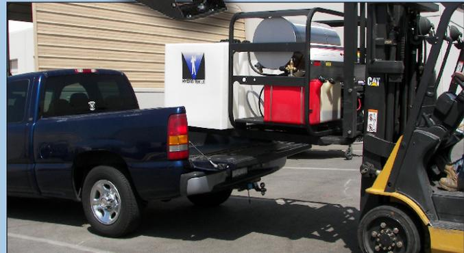
*Conveniently slides in (and out of) a full size truckbed and most flatbed or enclosed trailers. Skid, water tank and hose reels are plumbed and securely mounted to a steel powder coated tank skid. Saves time and hassle, just tighten bolts and go.*
