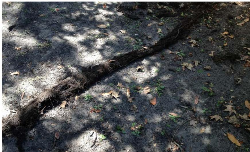
Photo of Root Ball Rucker pulled from the pool drainage pipes.
